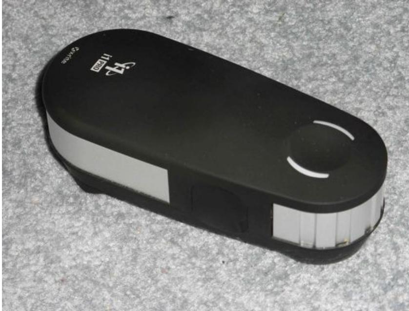
Figure 1: The X-Rite i1Pro2 Spectrophotometer
