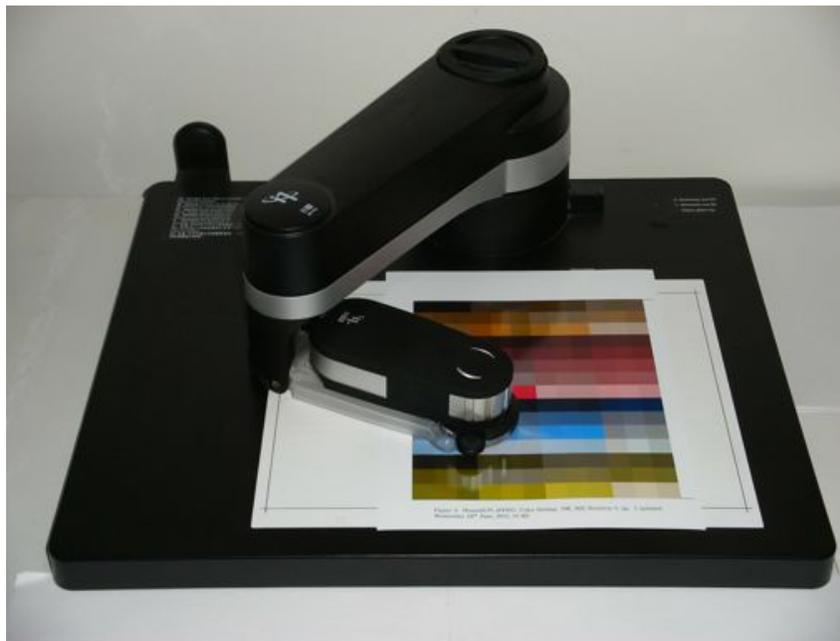
Figure 3: The X-Rite i1iO2 (an i1iO AST, equipped with an i1Pro2 spectrophotometer)
