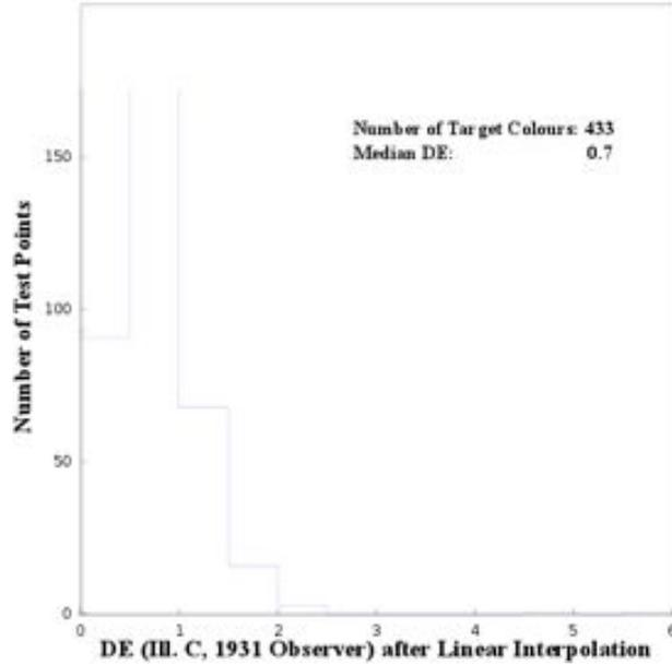
Figure 19: DEs to Linear Interpolants over a Set of 4096 RGBs
