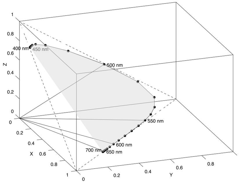
Figure 1: The  $XYZ$  Spectrum Cone, Cut by the Plane  $X + Y + Z = 1$
