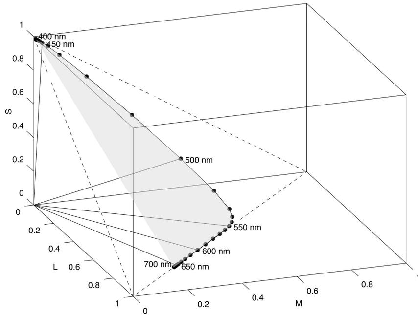
Figure 3: The *LMS* Spectrum Cone, Cut by the Plane  $L + M + S = 1$
