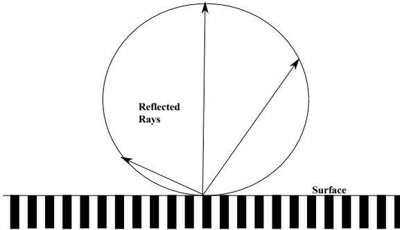
Figure 3.4: Lambertian Reflectance Distribution in a Plane Containing the Normal
