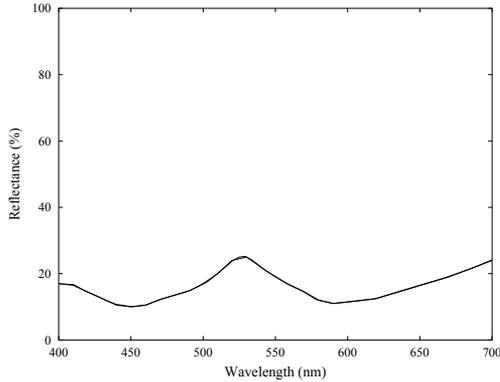
Figure 3.5: Reflectance Spectrum for Chromeoxide Green
