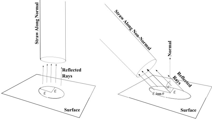
Figure 3.3: Reflected Rays in Different Directions
